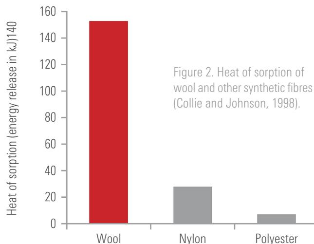
Figure 2. Heat of sorption of wool and other synthetic fibres (Collie and Johnson, 1998).
